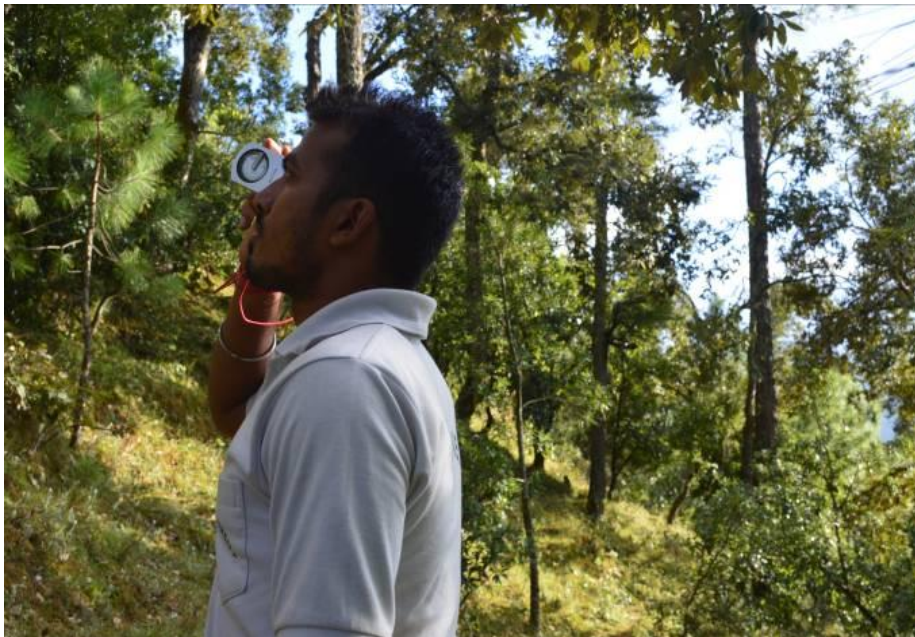
Fig 3. Tree height measurement using clinometer
